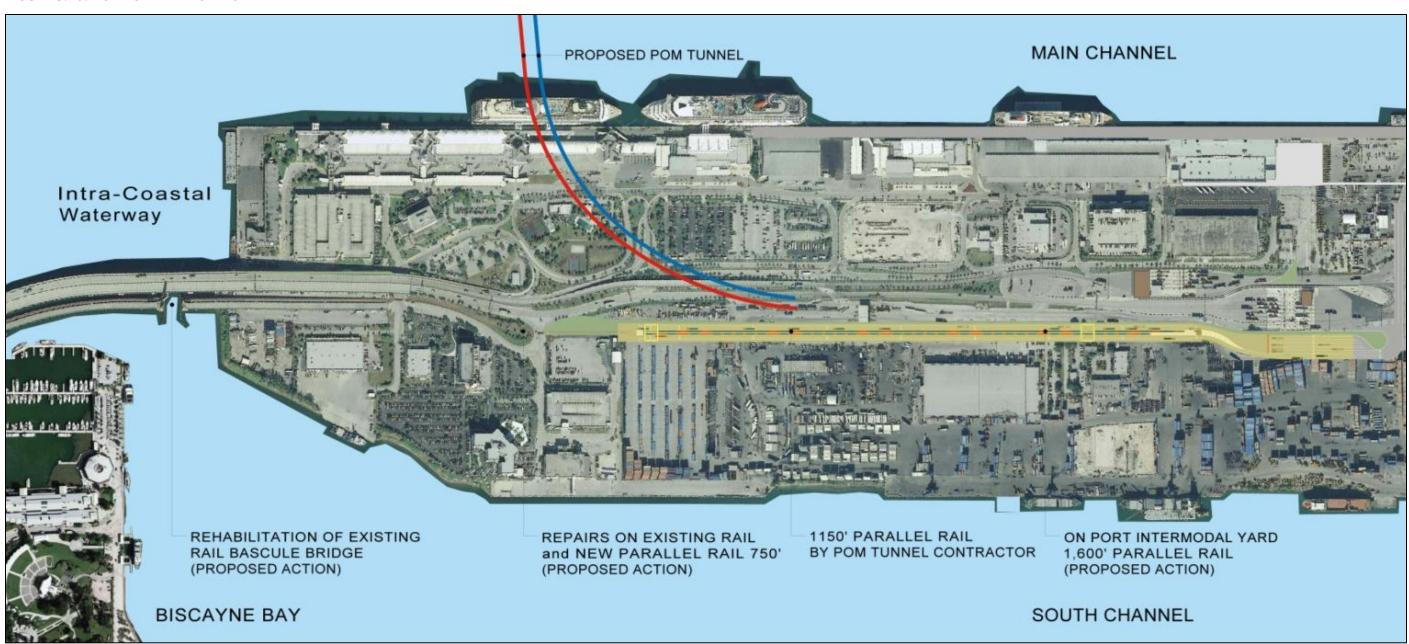
This rail yard would be used to stack and unload boxes from trains arriving and departing in the nighttime hours, thus not impacting downtown Miami traffic along Biscayne Boulevard. Aprons on either side would allow for loading/off-loading to occur. The existing bascule bridge would require substantial retrofitting prior to use. This is shown in the adjacent photo – Figure 5.21.
