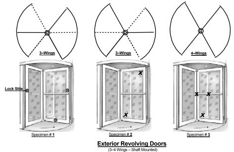
To qualify 2, 3 and 4 wings Revolving doors, test 2-wings sample #1 and samples #1 thru #3 from the 3 and 4 wings combination tests.
