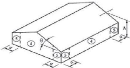
The width of zone 5 is the 'a' distance; it is either 10% of the least horizontal dimension of the structure - or - 0.4 times the mean roof height, but not less than 4% of the least horizontal distance -or- 3 feet. It is measured from the corner of the structure. Note that 3-feet is not the default value, it is the minimum width.
