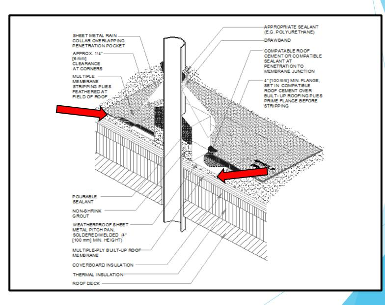
Pitch pans filled with roof cement are a poor choice for long term flashing penetrations, the roof cement will
