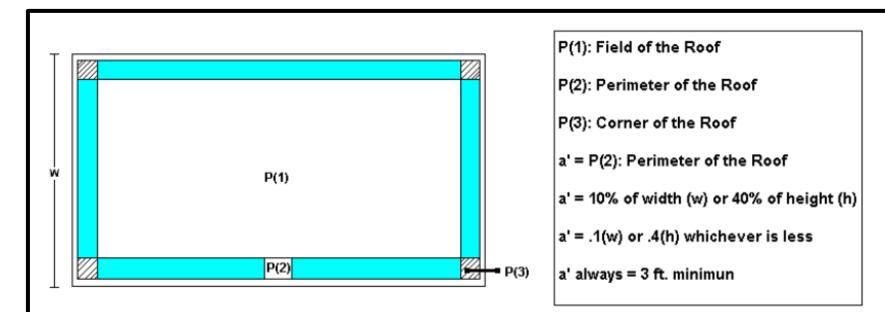
If a parapet equal to or higher than 3 ft. is provided around the entire perimeter of the roof then the uplift pressures of P(3) shall be equal to the uplift pressures of P(2).
