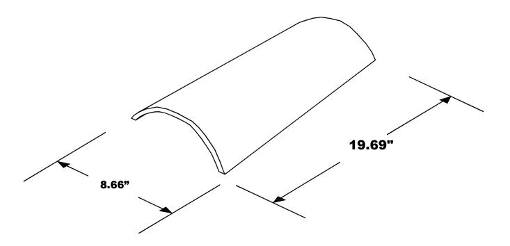
LA ESCANDELLA BARREL CLAY ROOF TILE
