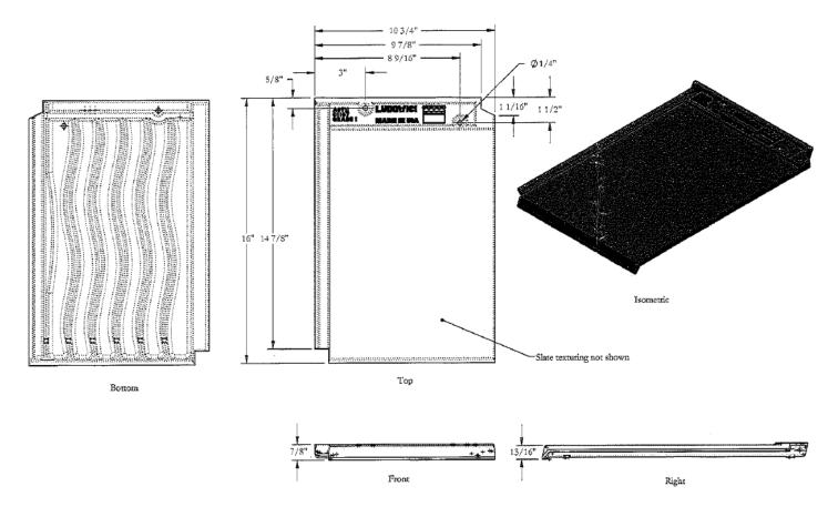
LUDO SLATE AND LUDO SHAKE CLAY ROOF TILE (LUDO SHAKE CONTAINS STRIATIONS ON TOP SURFACE TO RESEMBLE A WOOD SHAKE)
