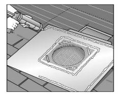
**2. SEAL** using sufficient amount Miami Dade approved sealant; Miami Dade approved ASTM D4586 Roof Cement (Class A where required by code for flame resistance) around inner and outer flange.
