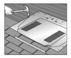
**4. SECURE** vent at 4-inch centers using roofing nails of sufficient length to penetrate sheathing. **SEAL** all penetrations using Miami Dade approved sealant (Class A where required by code for flame resistance). Miami Dade approved ASTM D4586 Roof Cement.
