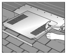
**5. COVER** with roofing material around vent. Based upon local best practices, a 45-degree angle cut may be made on the material terminating at the vent.
