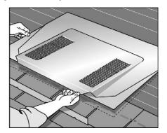
**3. PLACE** vent directly over 11-inch x 11-inch hole using previously marked outline as a guide.
