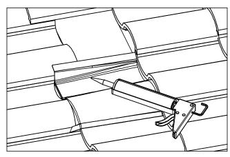
STEP 4: APPLY ROOFING SEALANT TO PILOT HOLES AND
