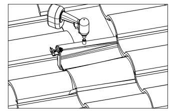
STEP 5: ATTACH THE BASE WITH (2) 5/16" LAG SCREWS, DRIVE LAG SCREWS FOR MINIMUM 2.5" EMBEDMENT INTO THE ROOF FRAMING MEMBER.
