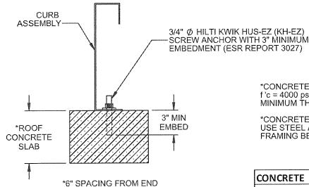
\*CONCRETE SLAB: f'c = 4000 psi MINIMUM NORMAL WEIGHT CONCRETE 6" MINIMUM THICKNESS, 12" MINIMUM EDGE DISTANCE
