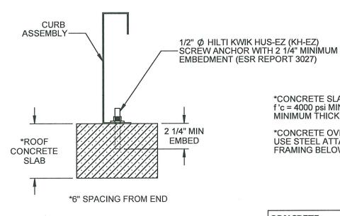
\*CONCRETE SLAB: f'c = 4000 psi MINIMUM NORMAL WEIGHT CONCRETE 5" MINIMUM THICKNESS, 12" MINIMUM EDGE DISTANCE
