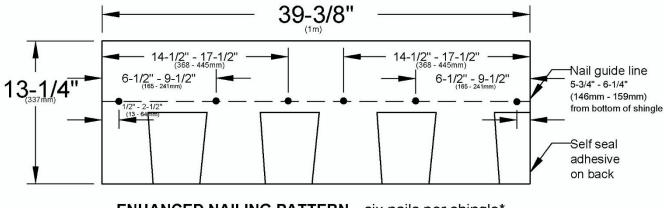
**ENHANCED NAILING PATTERN** - six nails per shingle\* \* required by some local codes and required for enhanced wind coverage on certain products. See limited warranty for details.
