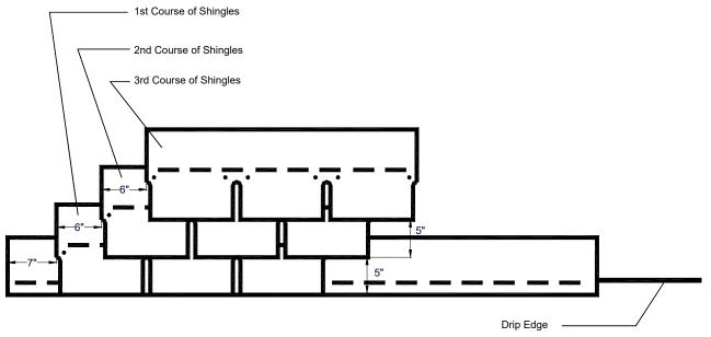
DETAIL B OVERALL DIMENSIONS AND NAILING PATTERN
