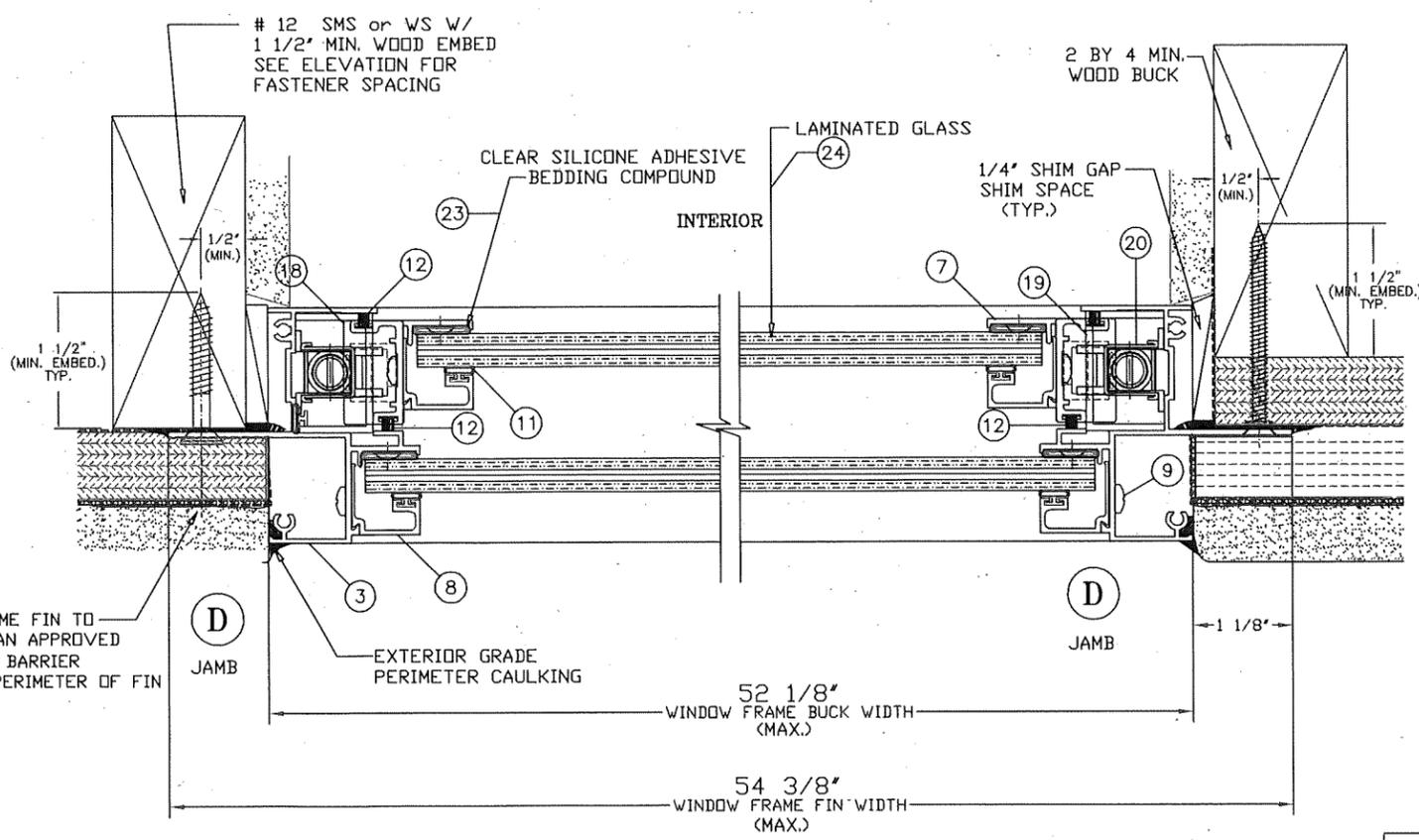
EXPOSED WINDOW FRAME FIN TO BE PROTECTED WITH AN APPROVED MOISTURE / WEATHER BARRIER THROUGHOUT ENTIRE PERIMETER OF FIN BY OTHERS (TYP.)
