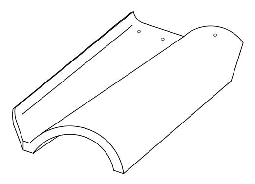
'S' CLAY ROOF TILE (DRAWING NOT TO SCALE)
