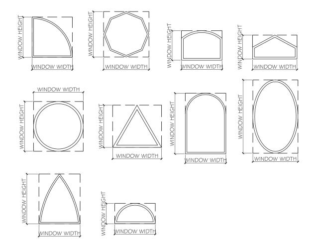
ALLOWABLE LOAD FOR ALTERNATE SHAPES AS SHOWN ABOVE OR SIMILAR CAN BE VERIFIED BY INSCRIBING PICTURE WINDOW SHAPE WITHIN SQUARE OR RECTANGLE AS SHOWN IN DOTTED LINES AND OBTAINING ALLOWABLE LOADS FROM THOSE SHAPES.
