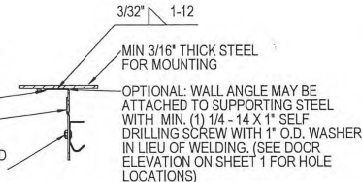
MOUNTING TO STEEL JAMB DETAIL
