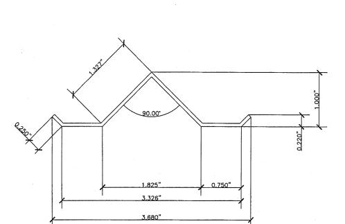
WALL THICKNESS = ,062" TYPICAL ALLOY = 6063TEMPER = T5MATERIAL = ALUMINUM
