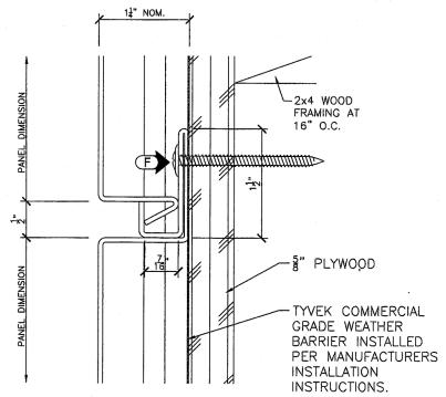
NOTE: FASTENERS MUST BE STAINLESS STEEL, FBC SECTION 2003.8.1.1.
