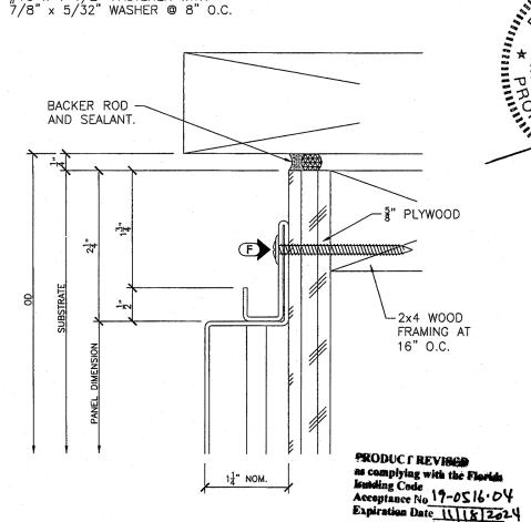
FASTENERS MUST BE STAINLESS STEEL, FBC SECTION 2003.8.1.1.
