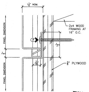
NOTE: FASTENERS MUST BE STAINLESS STEEL, FBC SECTION 2003.8.1.1. PRODUCT REVISED
