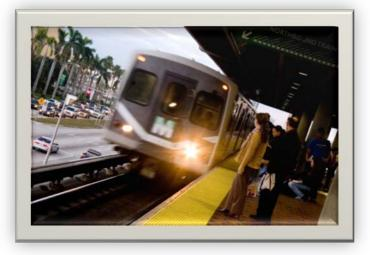
This project originally involved mid-life (15-year) rehabilitation of 136 Metrorail vehicles which is past due. The existing vehicles and subsystems are more than 20 years old and parts are becoming obsolete and more difficult to obtain. Fleet modernization will include rebuilding and/or replacement of existing components and systems with newer technology.
