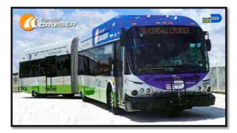
In June 2010 MDT implemented enhanced bus service operations with branded articulated diesel/electric hybrid buses, improved transit stops, Wi-Fi, Transit Signal Priority to communicate with traffic signal controllers that allows the equipped buses to save time at intersections while operating in mixed traffic, park-and-ride lots and improved headways. The Kendall Enhanced Bus Service (KEBS) is branded as the Kendall Cruiser featuring 22 stops along Kendall Drive over the 9-mile alignment from
