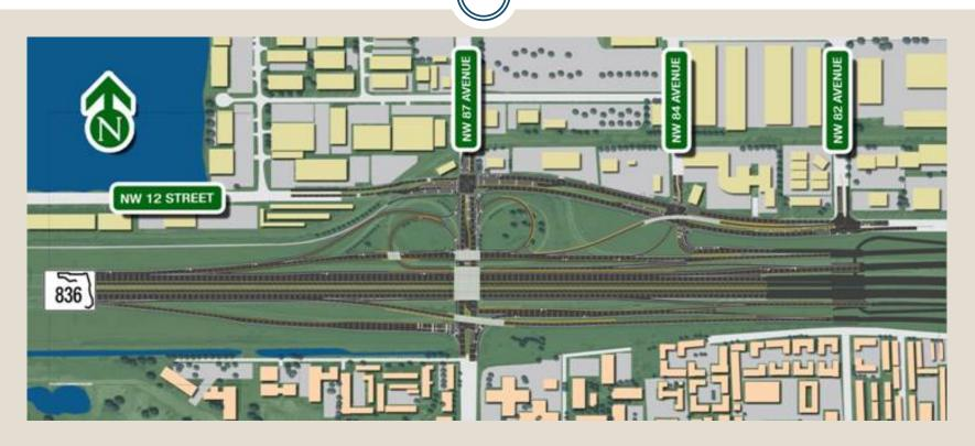
Improvements to SR 836 at NW 87<sup>th</sup> Avenue to provide system to system connection to SR 826 and increase capacity
