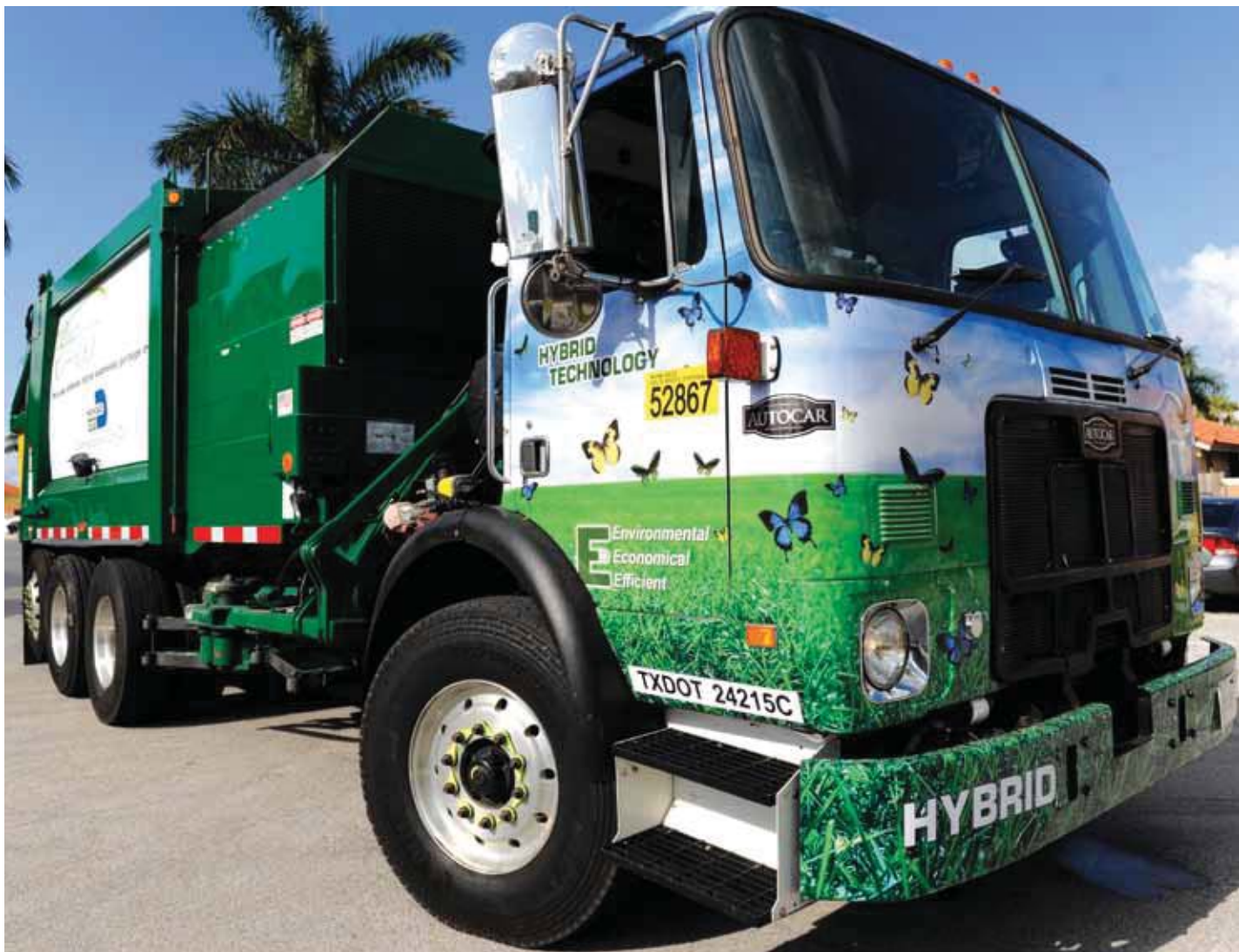
In September 2010, Miami-Dade County acquired the first of what is to become a fleet of six hybrid hydraulic diesel waste collection vehicles.
