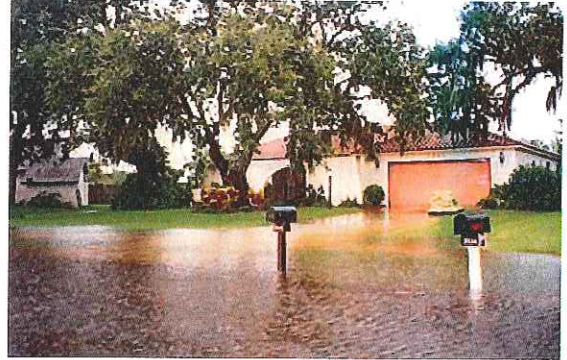
Figure 13: A flooded roadway stores excess run-off and protects neighboring houses.
