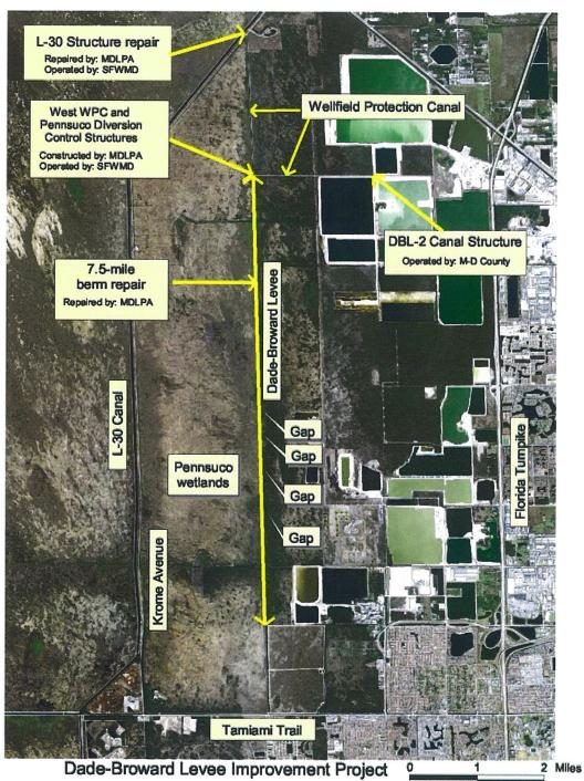
Project component (berm repair and water control structures) location map
