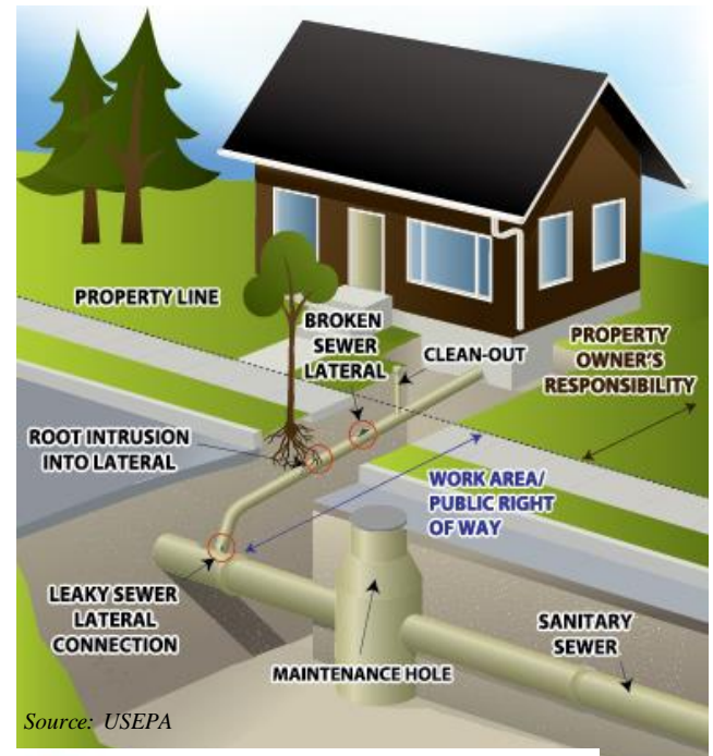
Figure 21: Key sources of inflow and infiltration (Source: EPA)
