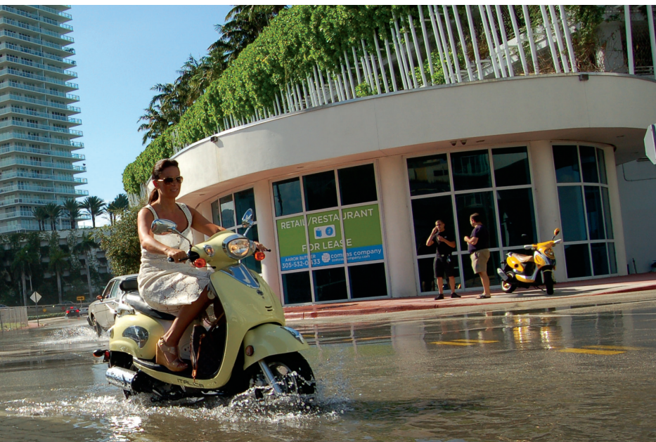
Flooding on Miami Beach on October 7, 2010 due to natural high tide exacerbated by on-shore winds, driving tidal waters up in to the streets through the stormwater drainage system.
