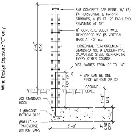
NOTE: CONCRETE BLOCK UNITS TO BE TYPE II—NONMOISTURE CONTROLLED, CONFORMING TO ASTM C90, WITH A MINIMUM NET AREA COMPRESSIVE STRENGTH OF 1900 PSI, (AVERAGE OF THREE). PRISM STRENGTH OF CMU WALLS F'm=1500 PSI.
