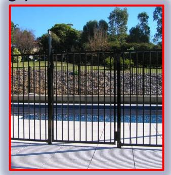
R4501.17.1.2 The barrier may not have any gaps, openings, indentations, protrusions, or structural components that could allow a young child to crawl under, squeeze through, or climb over the barrier as herein described below. One end of a removable child barrier shall not be removable without the aid of tools. Openings in any barrier shall not allow passage of a 4-inchdiameter (102 mm) sphere.
