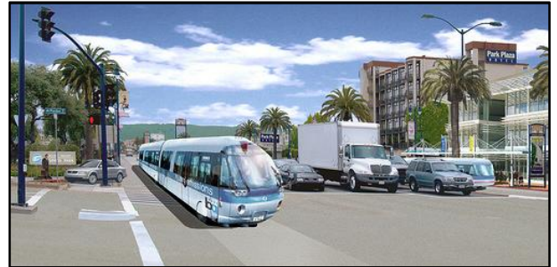
Visualization of queue jump operations illustrating a bus proceeding through an intersection ahead of general traffic
