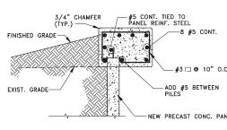
PLAN: ADDED REINF. @ PILES SCALE: 1/2" = 1'-0
