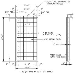
DETAIL: NON-TYPICAL PRECAST CONCRETE PANEL SCALE: 3/8" = 1'-0
