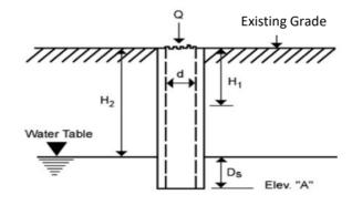
$$K = \frac{4Q}{\pi d (2H_2^2 + 4H_2D_8 + H_2d)}$$
