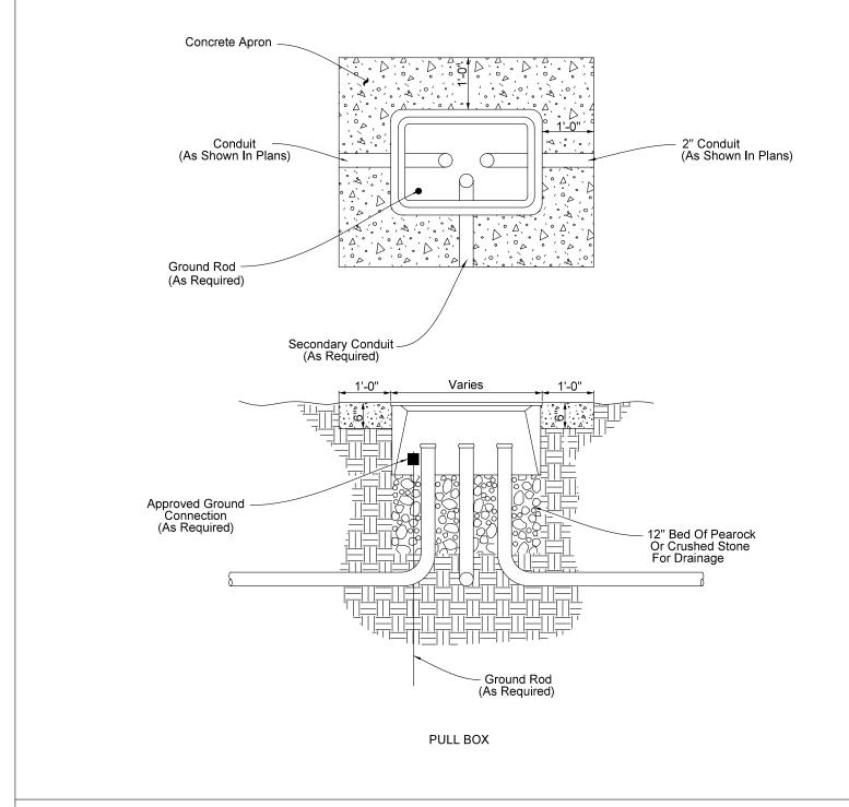
Conduit (As Shown In Plans) 2" Conduit (As Shown In Plans) Ground Rod (As Required) -Locate Wire (Typ) Secondary Conduit - Splice Box (200' Min.) Stored Fiber. Pull Box (50' Min.) Stored Fiber. (As Required) Varies 1'-0" \_1'-0"\_\_ Approved Ground Connection — Locate Wire- Locate Wire (As Required) 12" Bed Of Pearock Or Crushed Stone For Drainage Ground Rod (As Required) FIBER OPTIC BOX Rectangular boxes are depicted. Round fiber optic splice boxes and lids are allowed.
