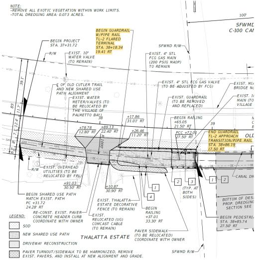
2. On the right hand side of the guardrail line it states to end guardrail with an approach transition. Could you clarify if a new wall will be constructed or will we be connecting to the existing wall (shown below).
