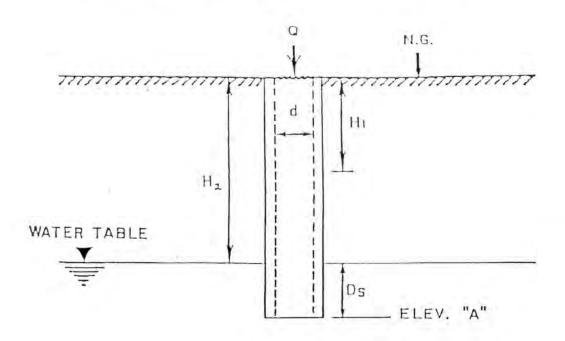
$$K = \frac{40}{\pi d(2H_2^2 + 4H_2D_S + H_2d)}$$
