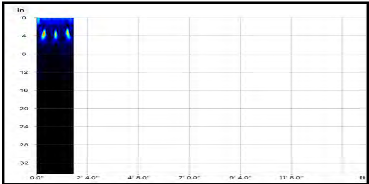
Column G:9 Longitudinal scan with Proceq GP8000. Present are three longitudinal bars. (H:9 similar)
