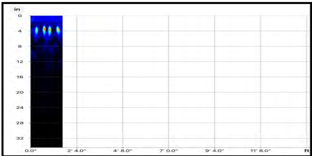
Column D:2 Longitudinal scan with Proceq GP8000. Present are 4 longitudinal bars. (D:4, D:15, D:17 similar)
