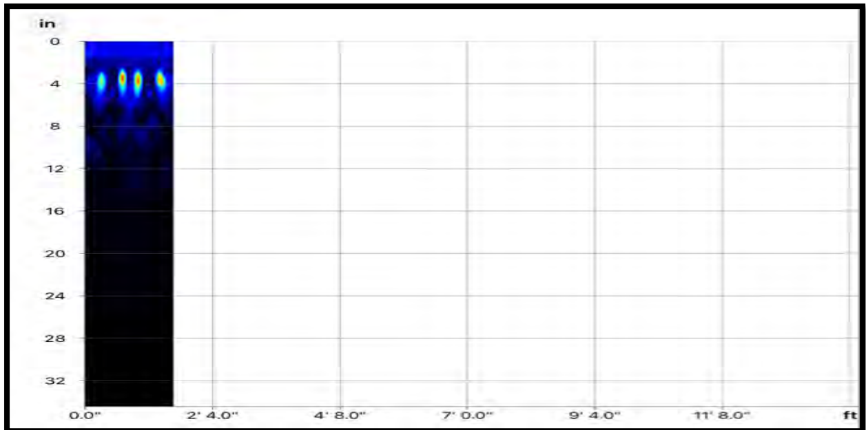
Column D:15 Shear scan with Proceq GP8000 from bottom to top. Four longitudinal bars are present. (D:17 similar)
