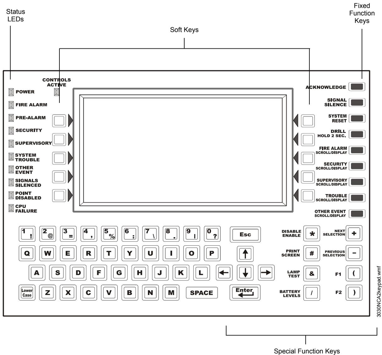
Figure 1.1 The Display/Keypad
