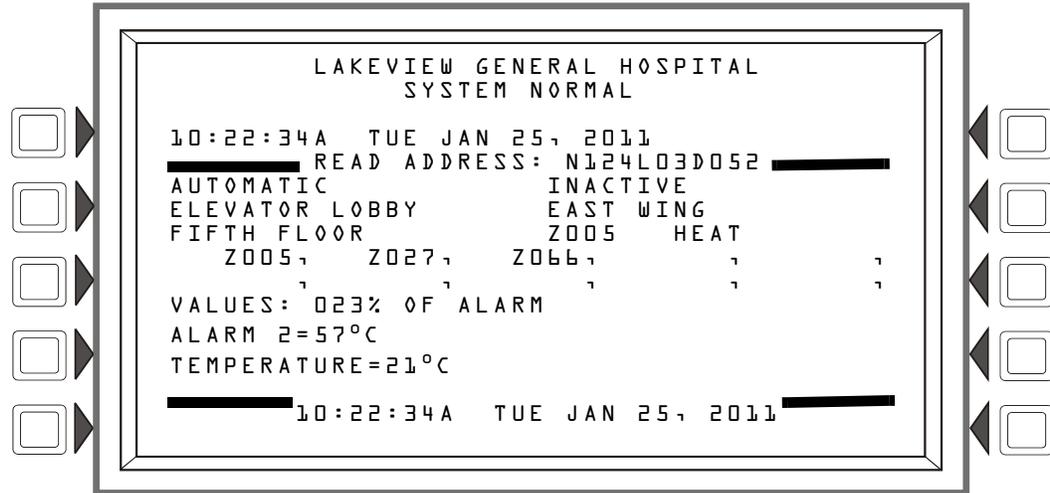
**Figure 3.3 Heat Detector Screen - Read Status**
