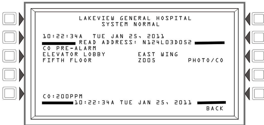
**Figure 3.5 Photo/CO Smoke Detector Screen (2) - Read Status**
