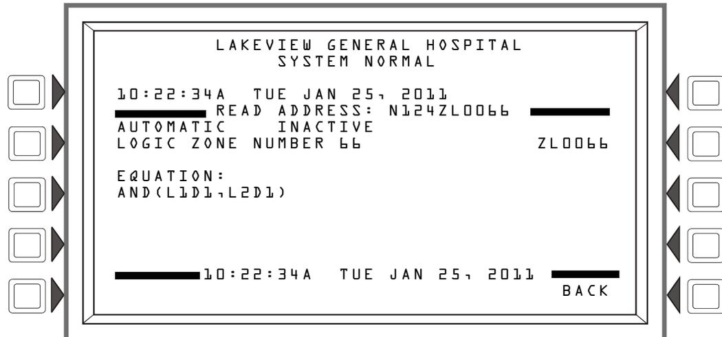
**Figure 3.9 Logic Zone Screen - Read Status**
