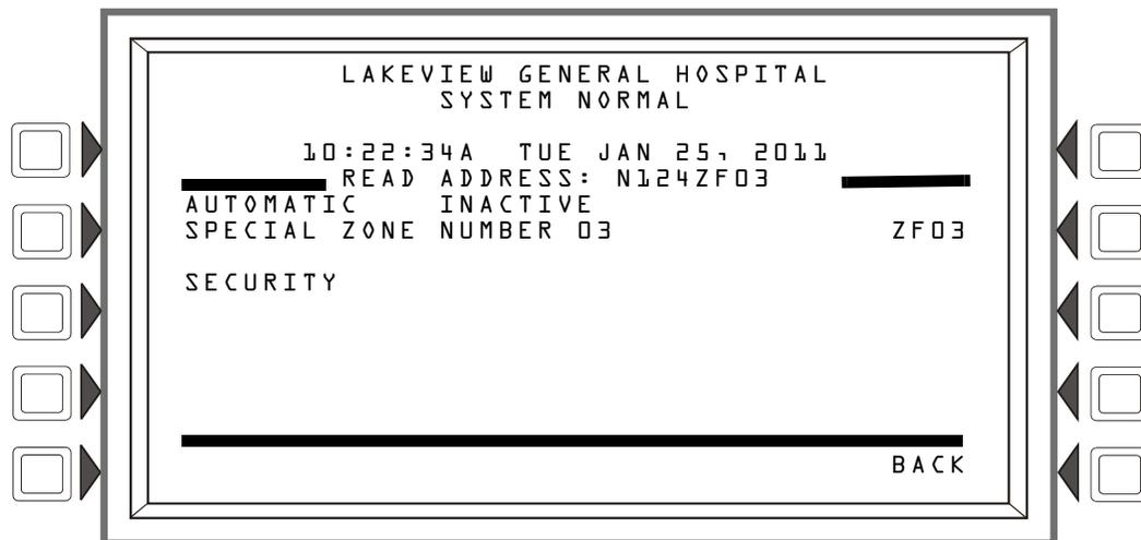
**Figure 3.11 Special Function Zone Screen - Read Status**
