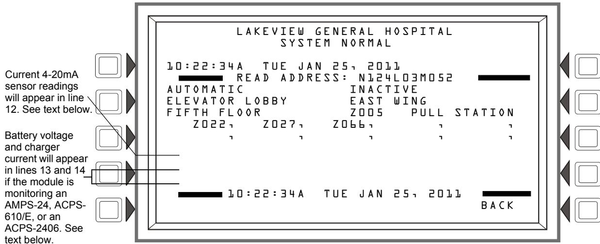
**Figure 3.6 Monitor Module Screen - Read Status**
