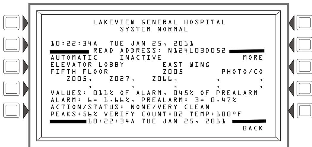
**Figure 3.4 Photo/CO Smoke Detector Screen - Read Status**
