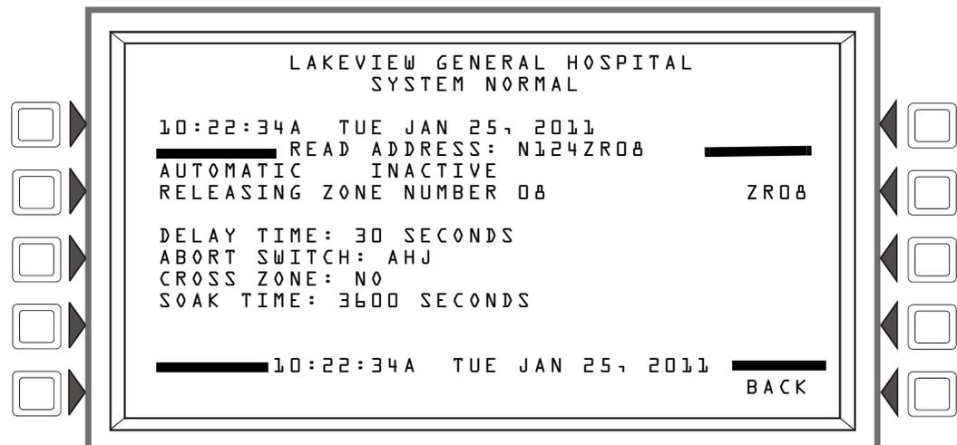
**Figure 3.10 Releasing Zone Screen - Read Status**
