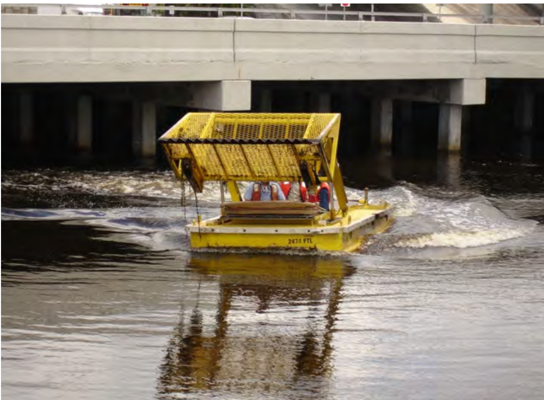
The bucket can push or collect the weeds, Water Hyacinth, and trash
