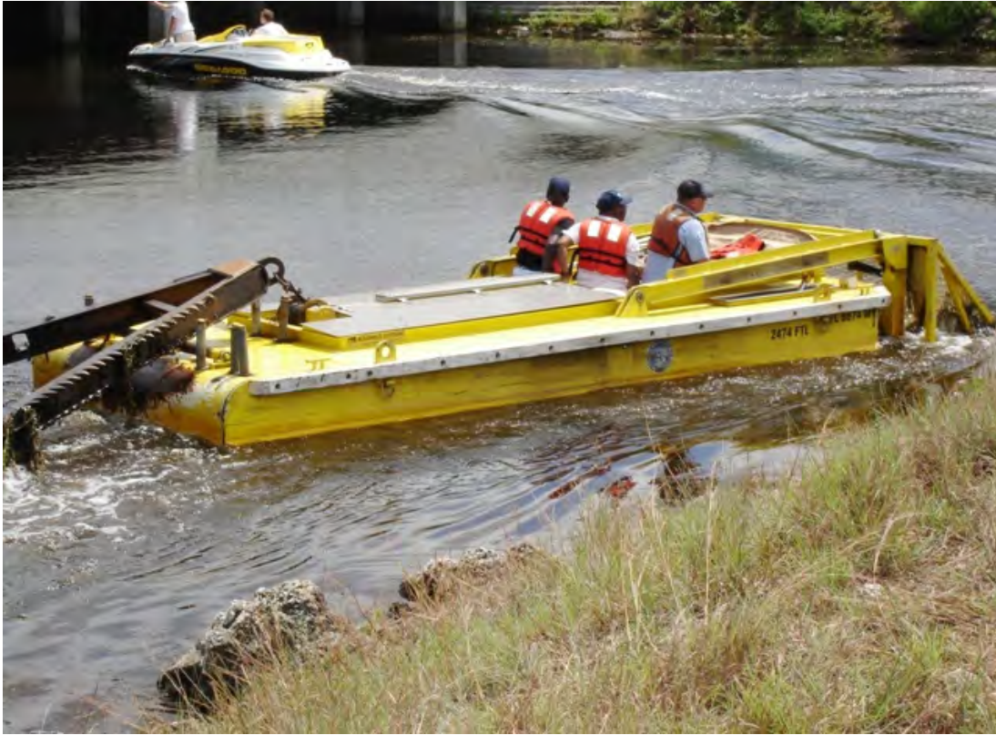
A plow is mounted on the back of the Weed Tow Boat
