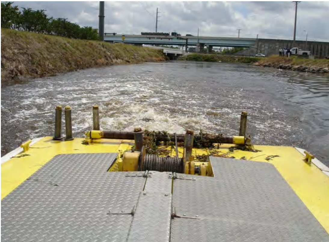
A winch lowers the plow into the canal
