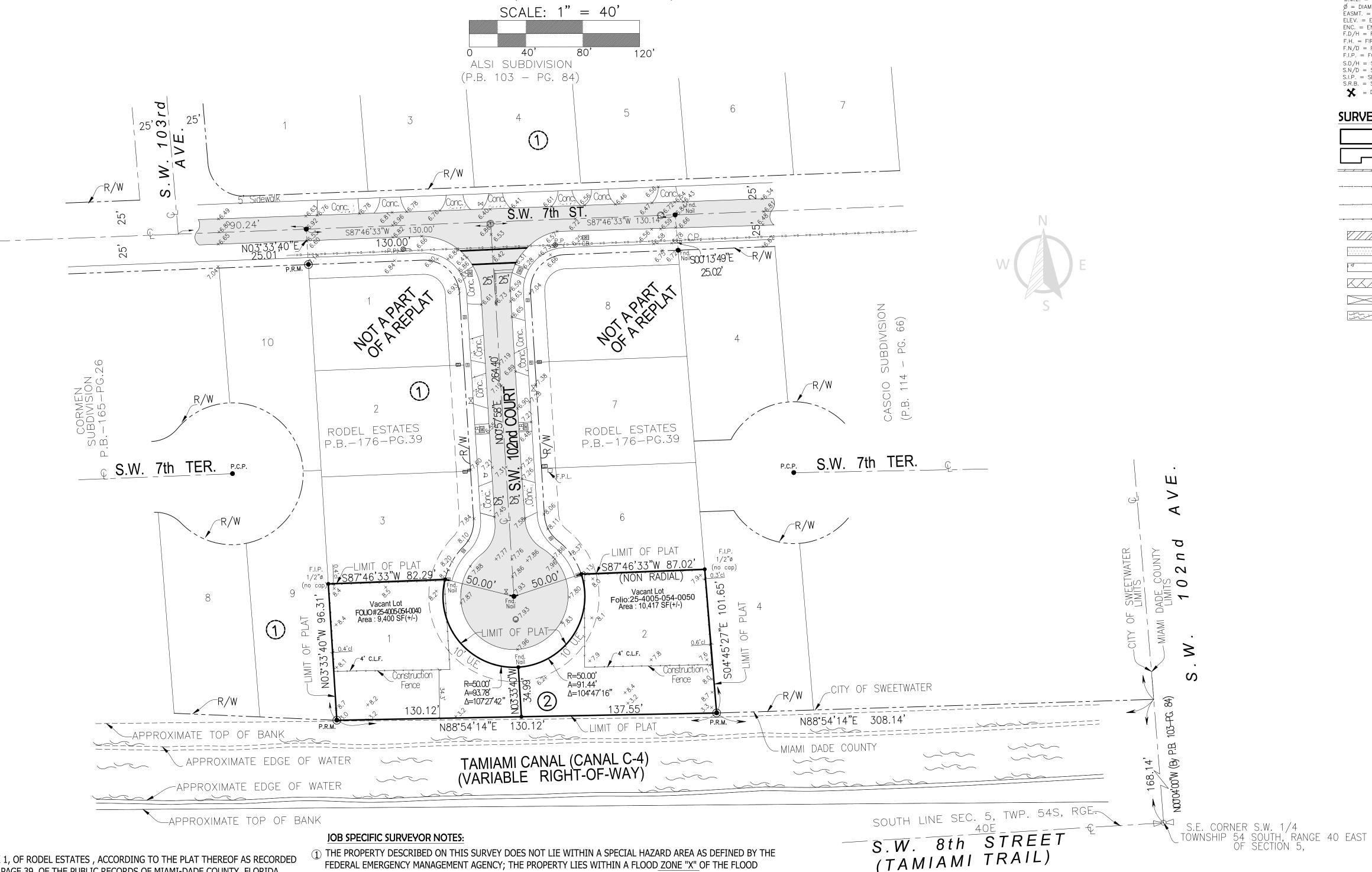
STY = STORY T.B.M. = TEMPORARY BENCH MARK A = CURVE LENGHT R = RADIUSL.P. = LIGHT POLE D = CURVE INTERIOR ANGLE MEAS.(M) = MEASUREDA/C = AIR CONDITIONING UNITMH = MANHOLEM = MEASUREDB.M. = BENCH MARK M = MONUMENT LINE NTS = NOT TO SCALE BIK/Corn.= BLOCK CORNER P/W = PARKWAYP.O.B. = POINT OF BEGINNING P.O.C. = POINT OF COMMENCEMENT P.C. = POINT OF CURVATURE
