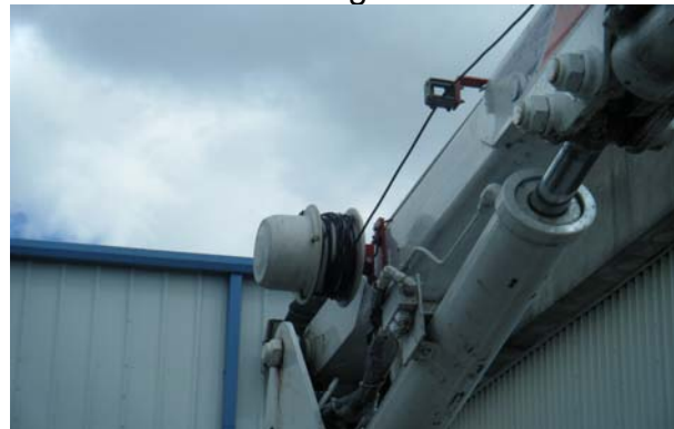
Cable Installed Along Crane Boom
