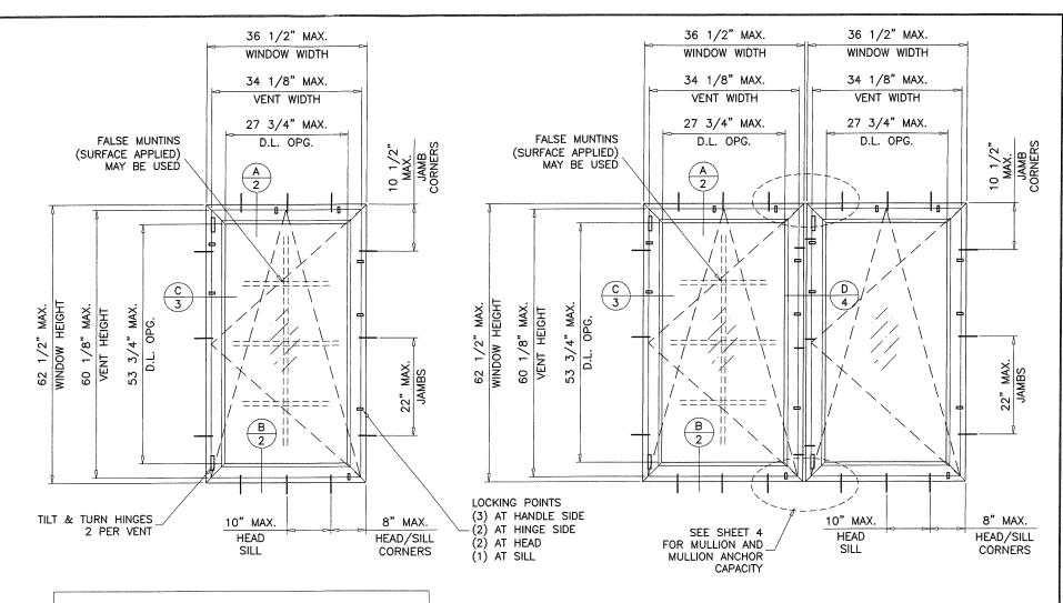
MAXIMUM DESIGN LOAD RATING = + 67.0 PSF (FOR SINGLE WINDOW SIZE SHOWN ABOVE 100.0 PSF OR SMALLER) SEE SHEET 4 FOR MULLION AND MULLION ANCHOR CAPACITIES.
