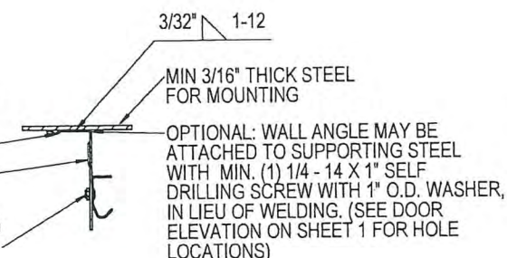
MOUNTING TO STEEL JAMB DETAIL
