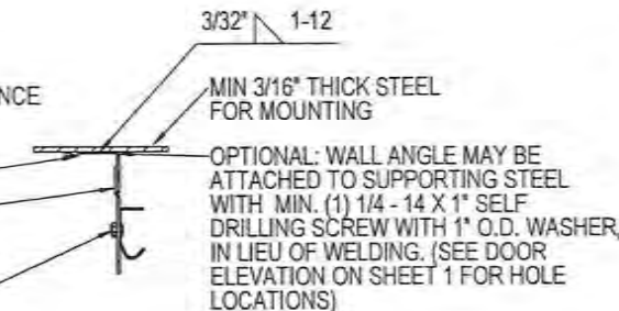
MOUNTING TO STEEL JAMB DETAIL
