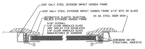
2. 3/16" X 1/2" SCREW - USED TO FASTEN THE STEEL EXTERIOR IMPACT WINDOW FRAME TO THE STEEL INTERIOR IMPACT WINDOW FRAME.
