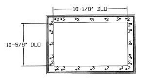
IMPACT GLAZING FASTENER DETAIL
