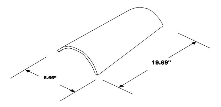
LA ESCANDELLA BARREL CLAY ROOF TILE
