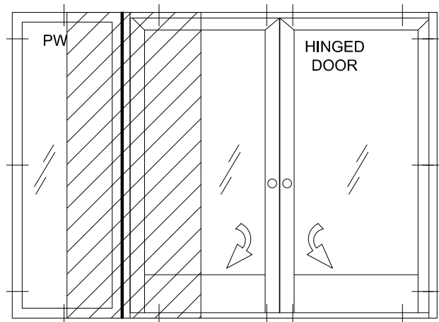
LOADING OF VERTICAL MULLION PANEL OF HINGED DOOR IS NOT CAPTURED OR ANCHORED
