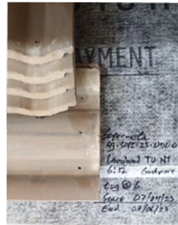
Figure 3: Profile with Lugs 6-tile stack (4 over 2)
