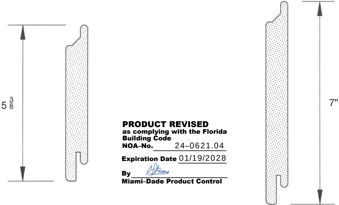
01 SECTION DETAIL - RAINCLAD SIDING (1x6) 1"= 2"
