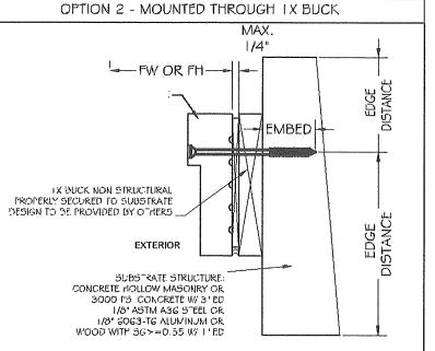
SUBSTRATE: MASONRY OR CONCRETE 1/4" TAPCONS BY ITW BUILDEX SECURING FRAME INTO SUBSTRATE WITH MAXIMUM 1/4' SHIM THROUGH IX
