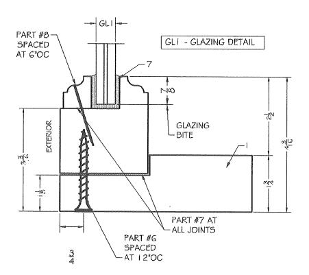
GLI-9/16" IMPACT GLASS COMPOSED OF: 1/4" HS OUTER LITE O. I O" GLASSLAM SAFETY PLUS II INTERLAYER 1/4" HS INNER LITE MINIMUM GLAZING BITE: 7/8"
