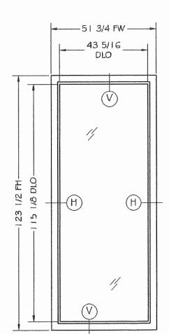
MODEL A ARCH FIXED WINDOWS (MAX, 123 1/2" X 51 1/4") DESIGNED LOADS PD= ±70 PSF
