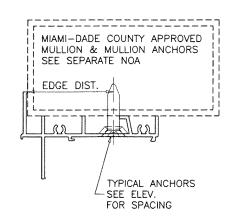
WOOD BUCKS AND METAL STRUCTURE NOT BY LABRADOR & FUNDORA CORP. dba-V & V WINDOWS MUST SUSTAIN LOADS IMPOSED BY GLAZING SYSTEM AND TRANSFER THEM TO THE BUILDING STRUCTURE.
