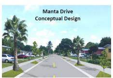
This project will consist of New sidewalks, ADA crosswalks, Driveway approaches, Continuous valley gutter, Improved drainage, Asphalt milling and resurfacing, Back of sidewalk harmonization, Street tree planting.
